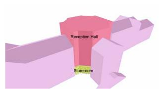
Figure 3: Each building block in the architectural information model is divided in different spaces, like for instance 'storeroom' and 'reception hall'.
